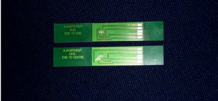
Example of FR4 Test PCB Used
